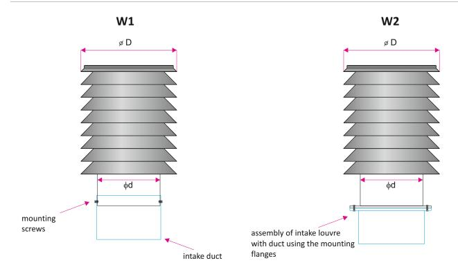
**Light type** - assembly visible with screws (louvre fitted onto duct)
