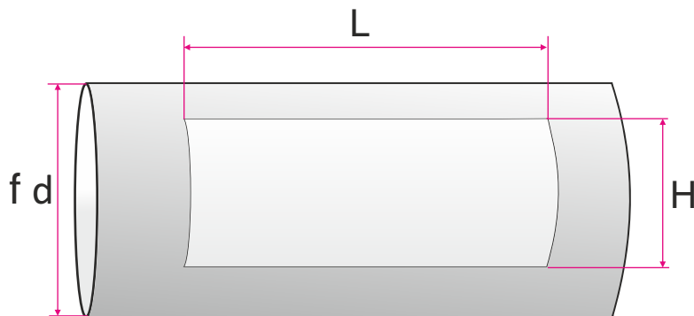
L,H - dimensions of the grille mounting hole
