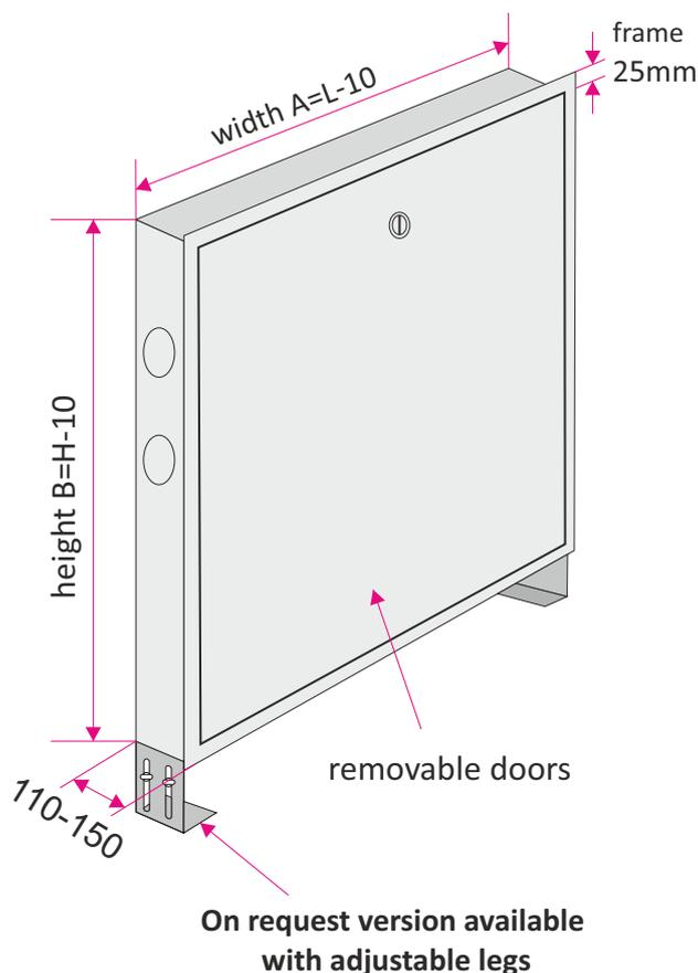
1. back part: box made of galvanized steel
